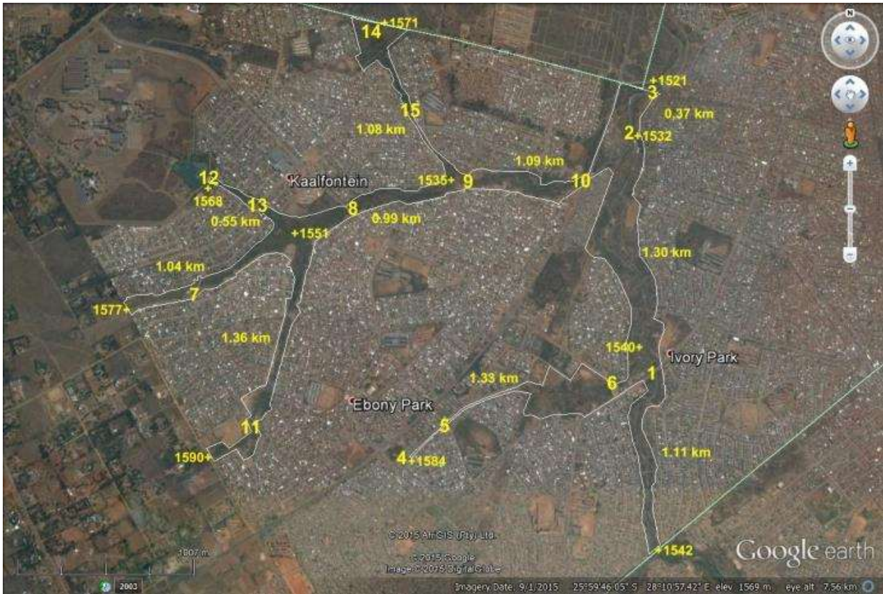
Figure 8: Sequence of positions for images taken to show the main features of each of the drainage systems involved along the mainstem Kaalspruit and its tributaries, starting each one upstream and ending downstream. Altitudes at points along the system are indicated as m a.s.l. (taken from Google Earth), and the straight-line distance between these points (+) as kilometres, to allow estimation of gradient. The estimated source of the Kaalspruit is at 1690 m a.s.l. and 7.37 km straight-line upstream of the study area.
